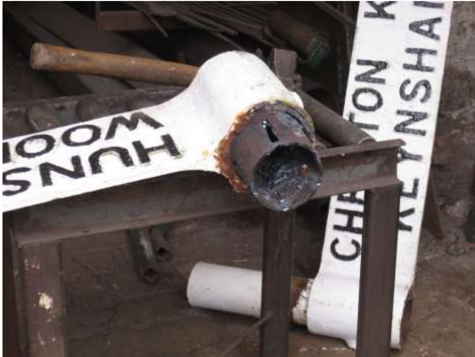
Rusted inner post exposed
