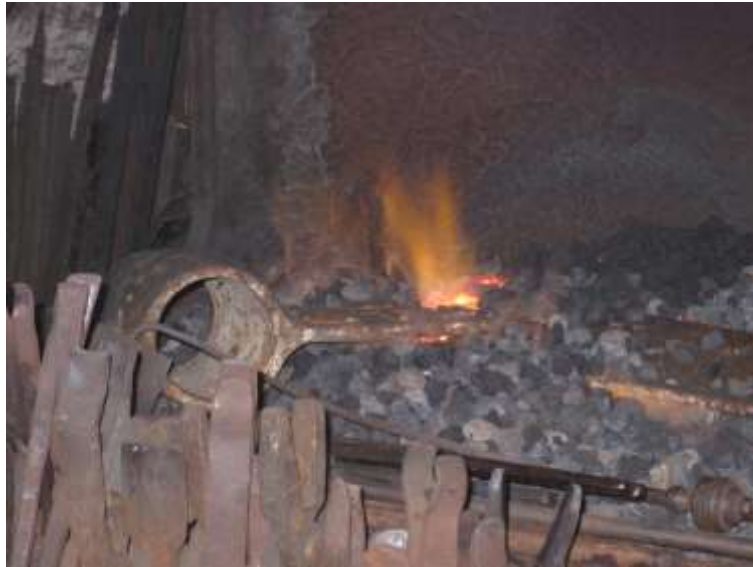
Preparing broken finger ready for welding
