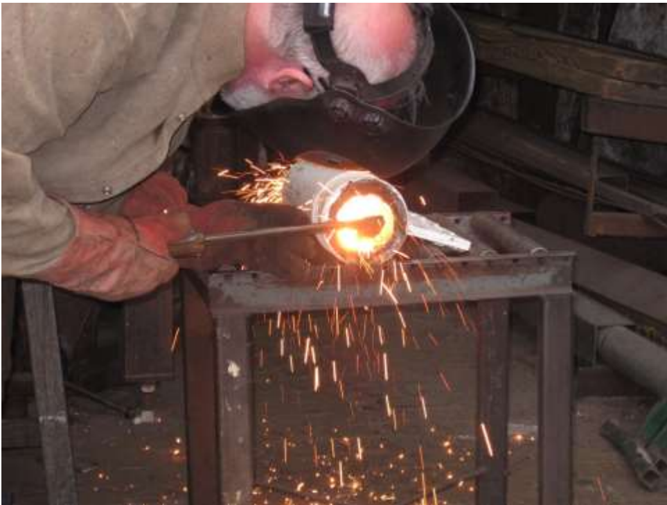
Gas cutting out rusted in inner post
