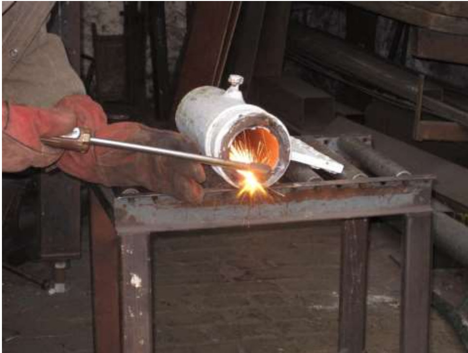
Gas cutting out rusted in inner post
