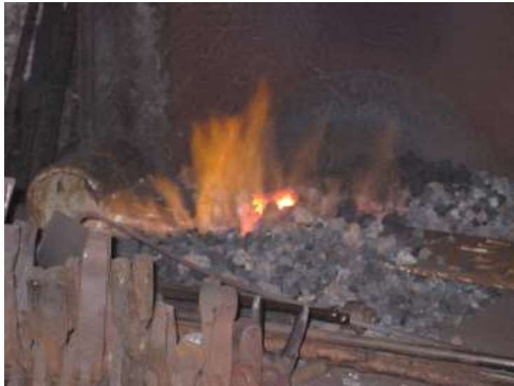
Preparing broken finger ready for welding
