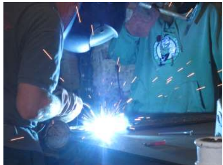
Arc welding to hold pieces together before the slower process of gas welding takes place
